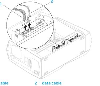
Press the release tabs together and slide the hard drive out of the hard 4. drive cage.
